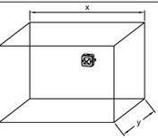
Category O-x-y (Open class): Centrally wall mounted, where x is the max height and width of the wall area covered by the device and y is the max depth of the volume covered by the VAD or ceiling mounted where x is the max width and length of the floor area covered of the VAD and y is the max ceiling height
