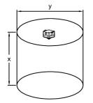
Category C-x-y (Ceiling mounted): Ceiling mounted, where x is the maximum ceiling height and y the diameter of the cylindrical volume covered by the VAD.
