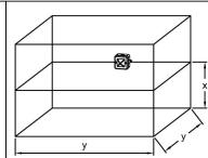
Category W-x-y (Wall mounted): Wall mounted, where x is the maximum mounting height from the floor and y is the maximum length of the sides of the square floor area covered by the VAD.
