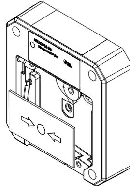
To fit the new glass element rotate the top cam clockwise by an angle of 50° (use a 6mm Allen key) this will then allow the glass to fit back into the pocket it sits in, resting on the pivot point and test cam, release the top cam to rest on the top of the glass element.
