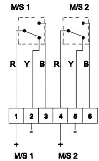
Unit in 'Operated condition' (broken glass)
