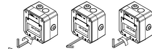
1. Insert test Key rotate clockwise 60°
