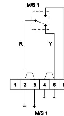
Unit in 'Operated condition' (broken glass)
