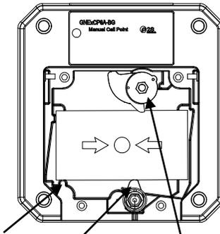
Pivot point Test Cam Top Cam (rotate)
