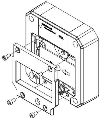
Once the cover is removed the broken glass will be free to be removed, clean out any other fragments of glass carefully.
